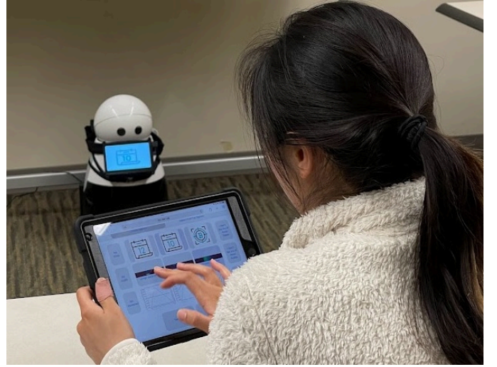
Fig. 3. Customization session setup. Participant designing signals for the modified Kuri robot using the query-based interface.
